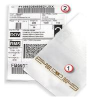
When an RFID tag comes within range of an antenna, the unique electronic product code (EPC) within the RFID tag is read automatically, and then translated by the RFIDBox into the movement of the container or item, to which the Tag is attached, to the location (such as a work-station) where the antenna is.
