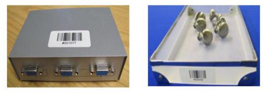
When a batch of individually tagged work-in-process is to be tracked, the process starts out by printing out the barcode/RFID tags, one for each item to be tracked. This also results in an entry for each item being created in the containers table in the BellHawk, which is associated with the work order and/or customer order for which these items are intended.
