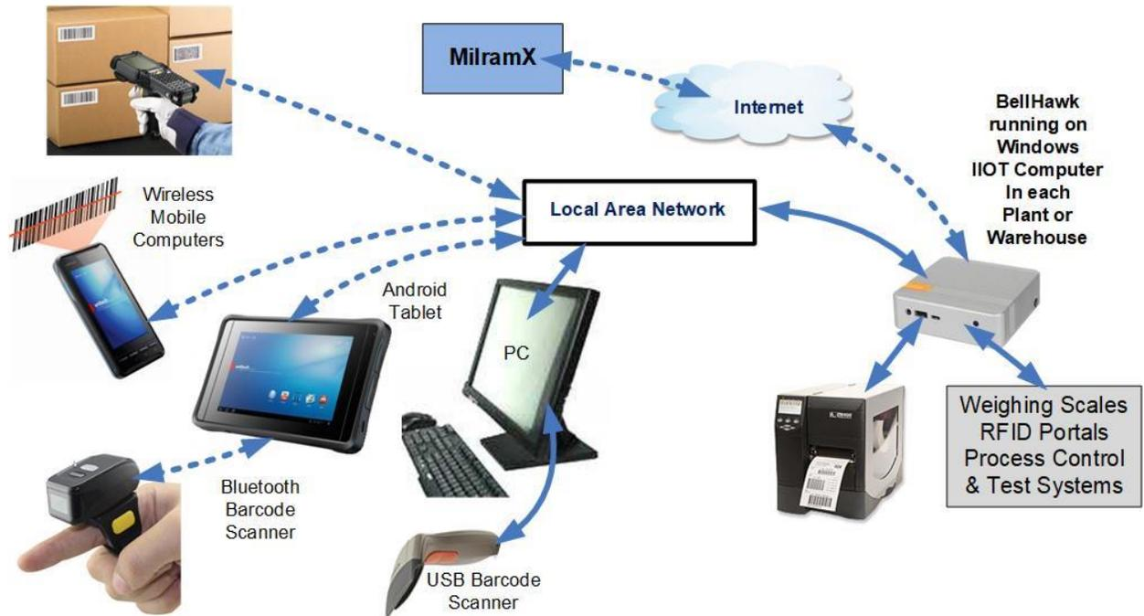
Here the BellHawk system, implemented in the Pilot, is installed in a ruggedized industrial computer so that it can run 24x7 without any risk of Internet or Cloud-computing failure interrupting operations.
