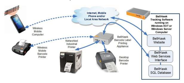
The BLPA is a ruggedized IIOT (Industrial Internet of Things) computer, which is shipped to each site, complete with all the needed label printing software, ready to plug in.
