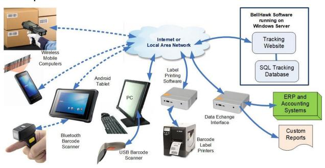
The BellHawk software consists of a specialized website and a SQL server database, which run on a Windows Server computer. This software can be installed at a client's own data center or
